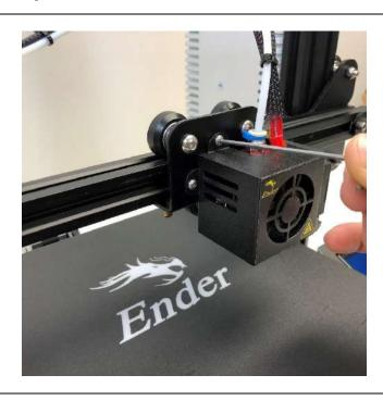
Use the 2mm Allen wrench to remove the fan shroud
