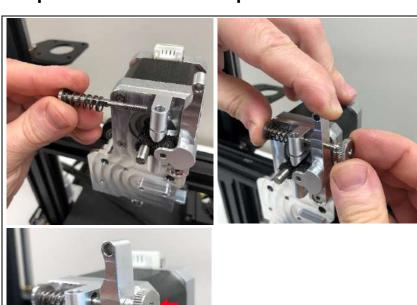
Screw in the lever adjusting knob until the pin is flush with the knob.
