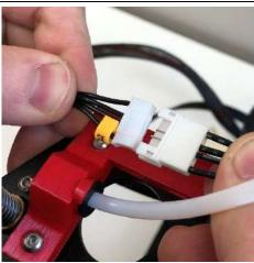
Connect the extruder motor with the provided custom extension cord
